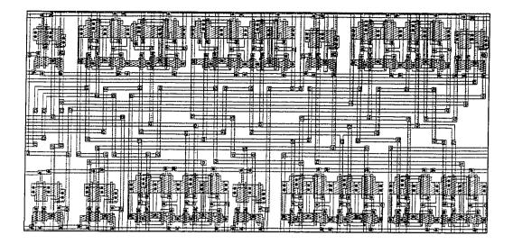
**Figure C-6** Routing (C132): 426x201λ, 5.3k
