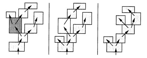
Figure 3-13 Two Subtrees Orphaned by a Tile Deletion
