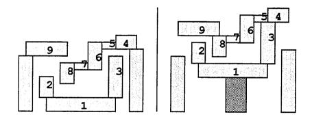
Figure 3-2 Tile Insertion Movement Order
