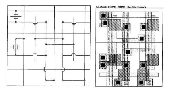
Figure 1-1 RAM Cell Stick Diagram and Layout
