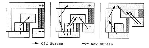
Figure 3-8 Stress Reduction: Three Added Stress Paths
