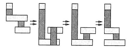
Figure 2-12 Fixing Negative Length Wires
