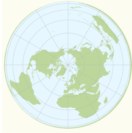
Figure 4.6: Example of equal-area Lambertian projection to “flatten” the North hemisphere into a disk. In order to preserve area the projection map has to distort angles, which affects the shapes close to the equator.
