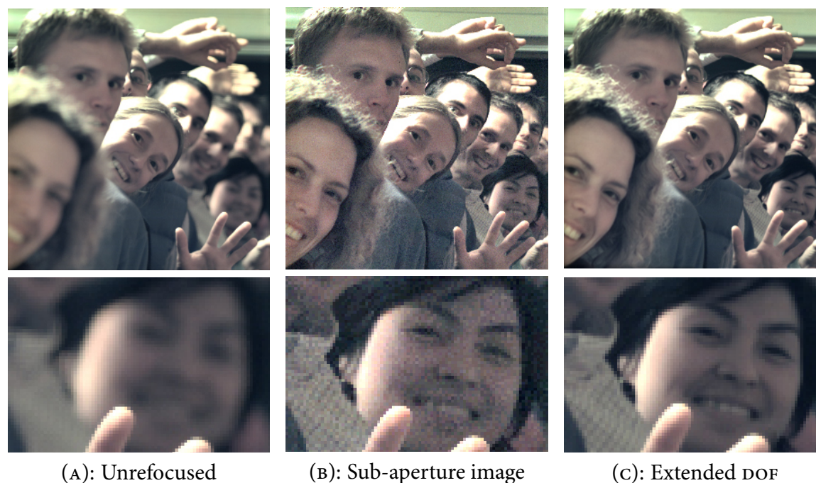
Figure 4.4: Comparison of a sub-aperture image and an image computed with digitally extended depth of field.
