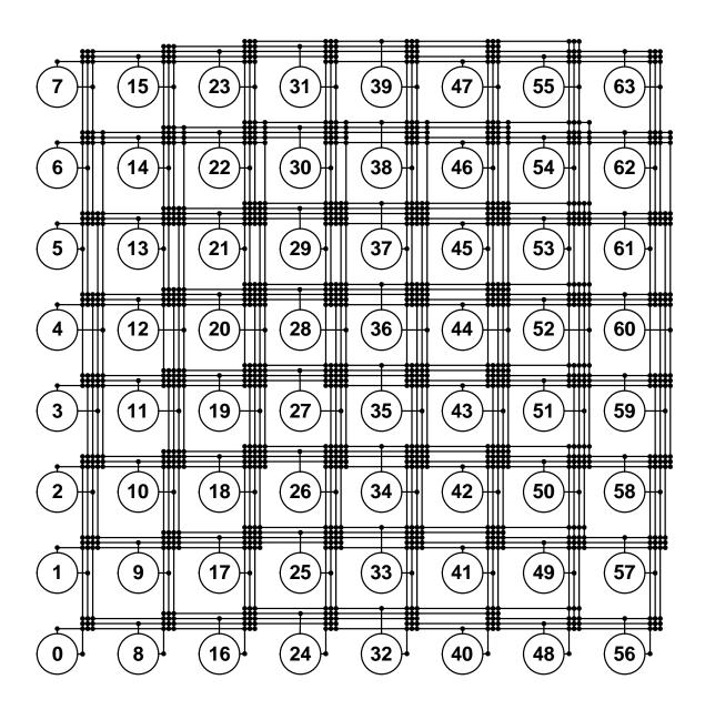
Figure 7.13: Limited-Connectivity Inercluster Switch for 8x8 Cluster Floorplan
