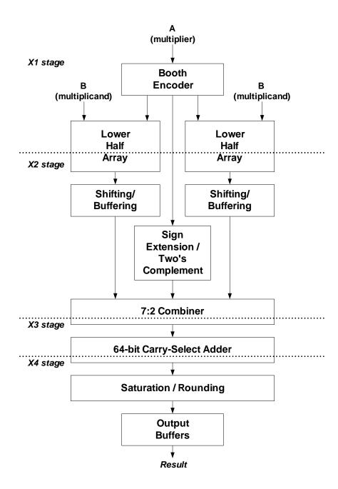
Figure 3.12: MUL Unit Block Diagram
