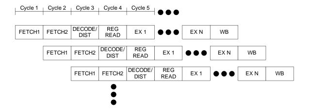
Figure 3.6: Kernel Execution Pipeline Diagram
