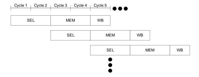
Figure 3.8: SRF Pipeline Diagram
