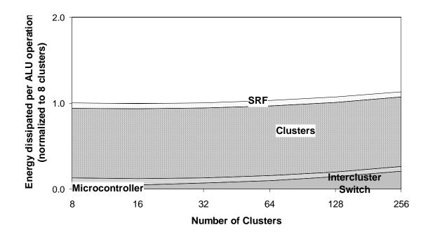
Figure 6.6: Energy of Intercluster Scaling
