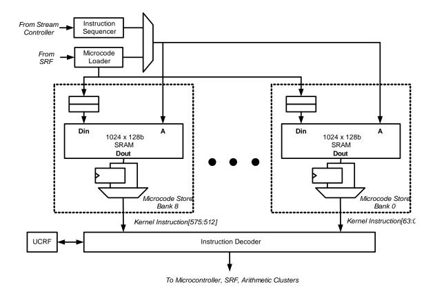
Figure 3.3: Microcontroller Block Diagram
