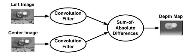
Figure 2.1: A Stereo Depth Extractor
