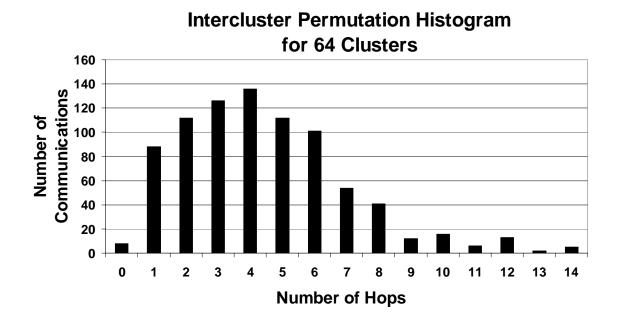
Figure 7.12: Intercluster Switch Locality with 8x8 Cluster Grid Floorplan
