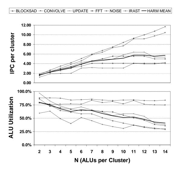
Figure 7.4: Intracluster Scaling with Software Pipelining
