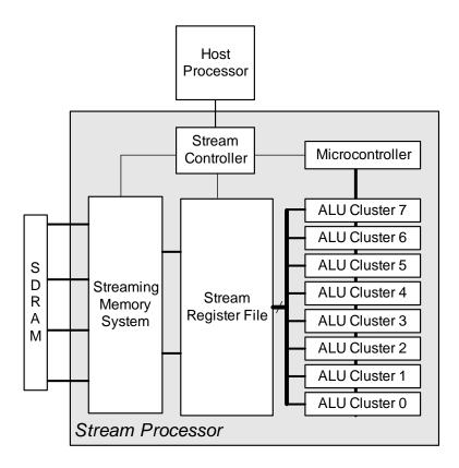
Figure 2.3: Stream Processor Block Diagram
