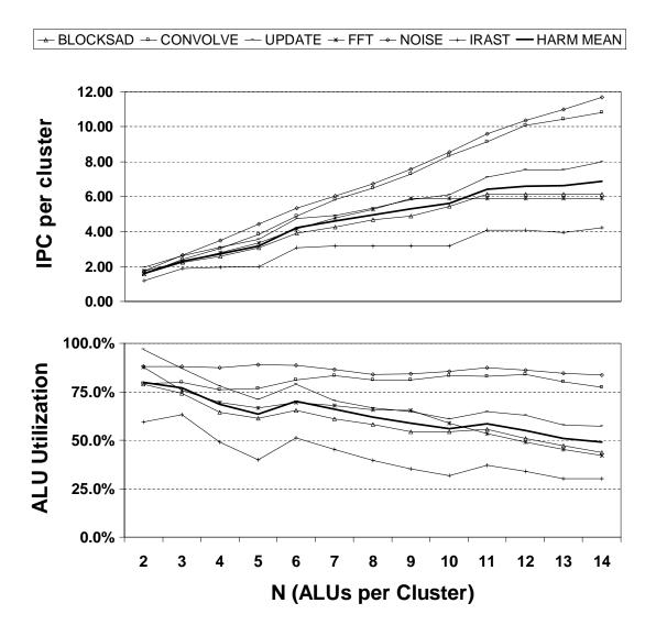
Figure 7.5: Intracluster Scaling with Software Pipelining and Loop Unrolling
