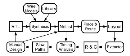
Figure 4.1: Standard ASIC Design Methodology
