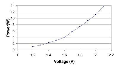
Figure 5.4: Measured Core Power Dissipation
