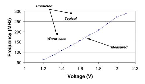
Figure 5.2: Measured Operating Frequency
