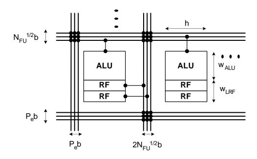
Figure 6.2: Intracluster Switch Floorplan
