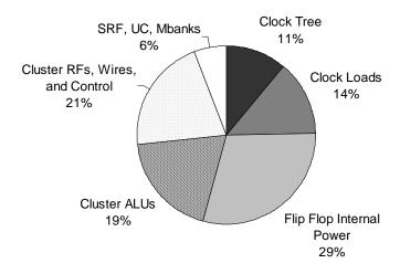
Figure 5.5:  $C_{sw}$  distribution during Active Operation
