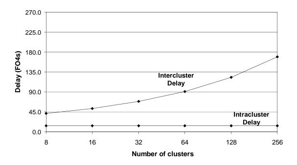
Figure 7.2: Worst-case Switch Delay with Intercluster Scaling
