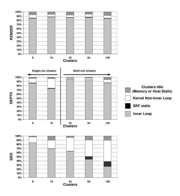
Figure 7.10: Application Cycles with Intercluster Scaling (N=5)
