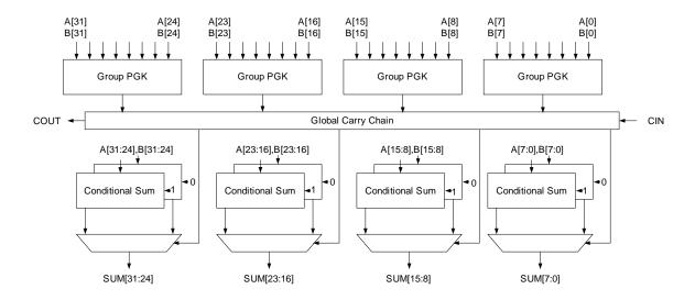
Figure 3.11: Segmented Carry-Select Adder
