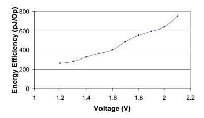
Figure 5.6: Measured Energy Efficiency
