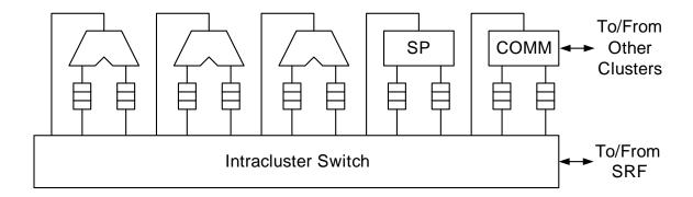
Figure 2.4: Arithmetic Cluster Block Diagram
