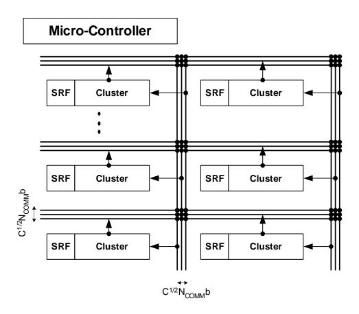
Figure 6.1: Scalable Grid Floorplan
