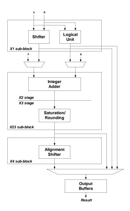
Figure 3.10: ALU Unit Block Diagram
