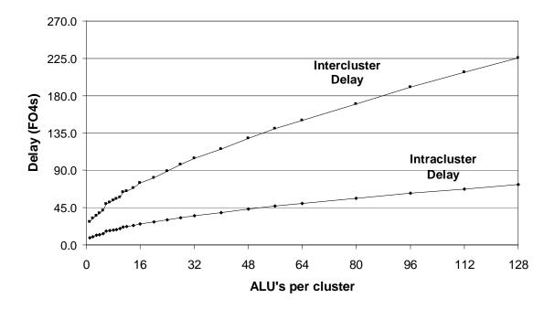
Figure 7.1: Worst-case Switch Delay with Intracluster Scaling
