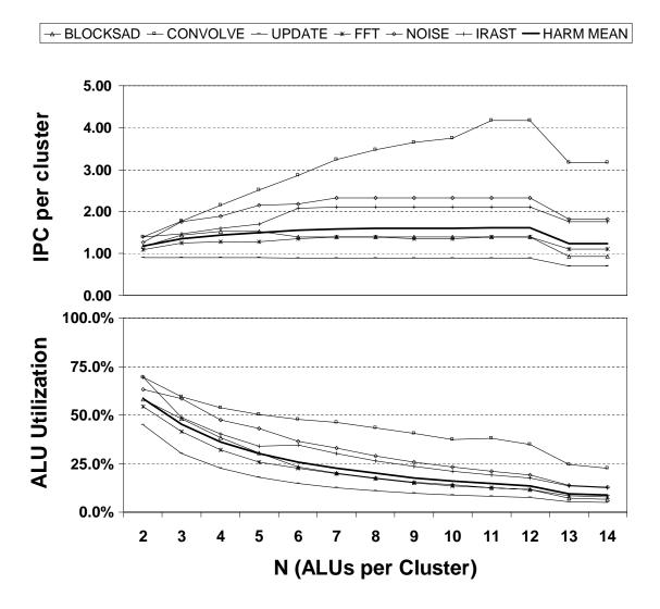
Figure 7.3: Intracluster Scaling with no Loop Transformations
