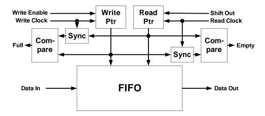
Figure 4.4: Asynchronous FIFO Synchronizer
