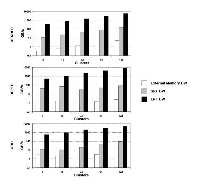
Figure 7.11: Bandwidth Hierarchy with Intercluster Scaling (N=5)
