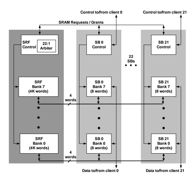
Figure 3.7: Stream Register File Block Diagram
