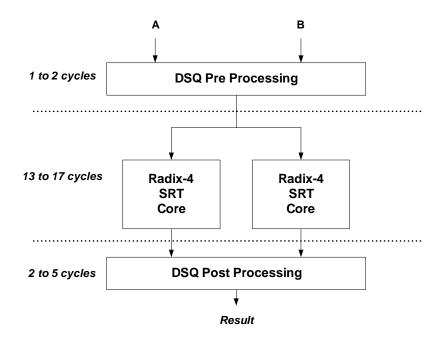
Figure 3.13: DSQ Unit Block Diagram
