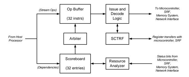
Figure 3.9: Stream Controller Block Diagram
