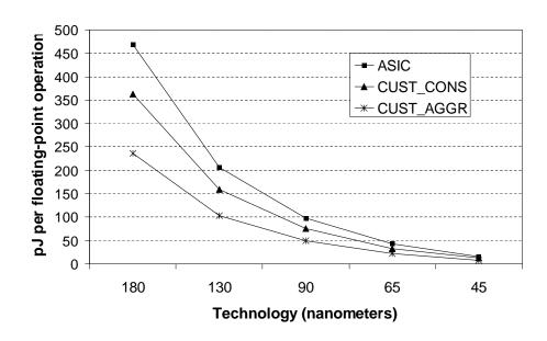
Figure 6.9: Effect of Technology Scaling on Energy Efficiency
