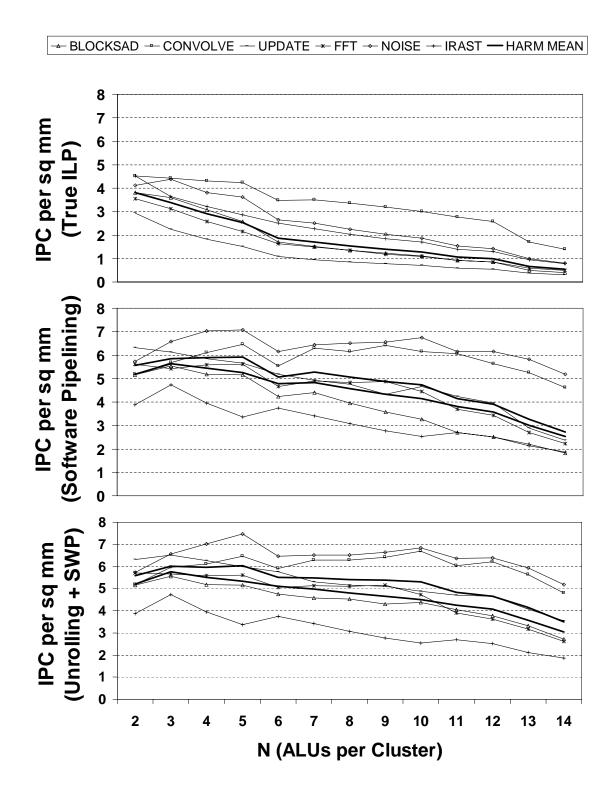
Figure 7.6: Inner-Loop Performance per Area with Intracluster Scaling
