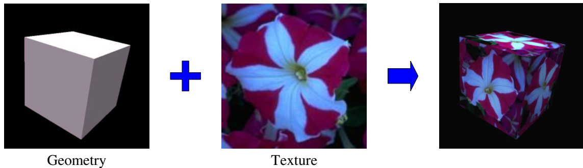
Figure 2.3: The cube on the left is texture mapped with the image of the flower. The result is shown on the right.
